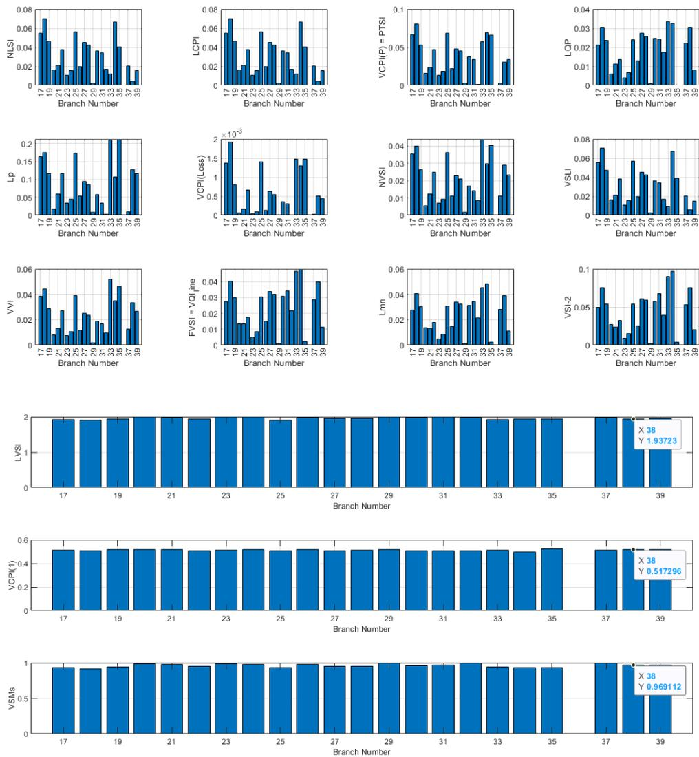
Figure 6.22 VSIs of all 33 kV transmission lines, PL = 5%, type3 DG.
