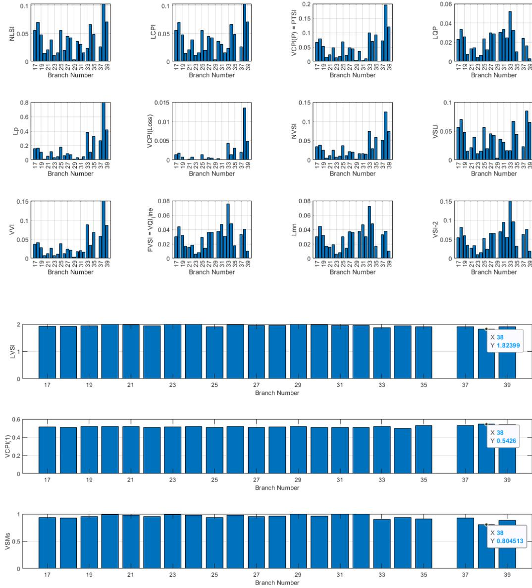
Figure 6.23 VSIs of all 33 kV transmission lines, PL = 10%, type3 DG
